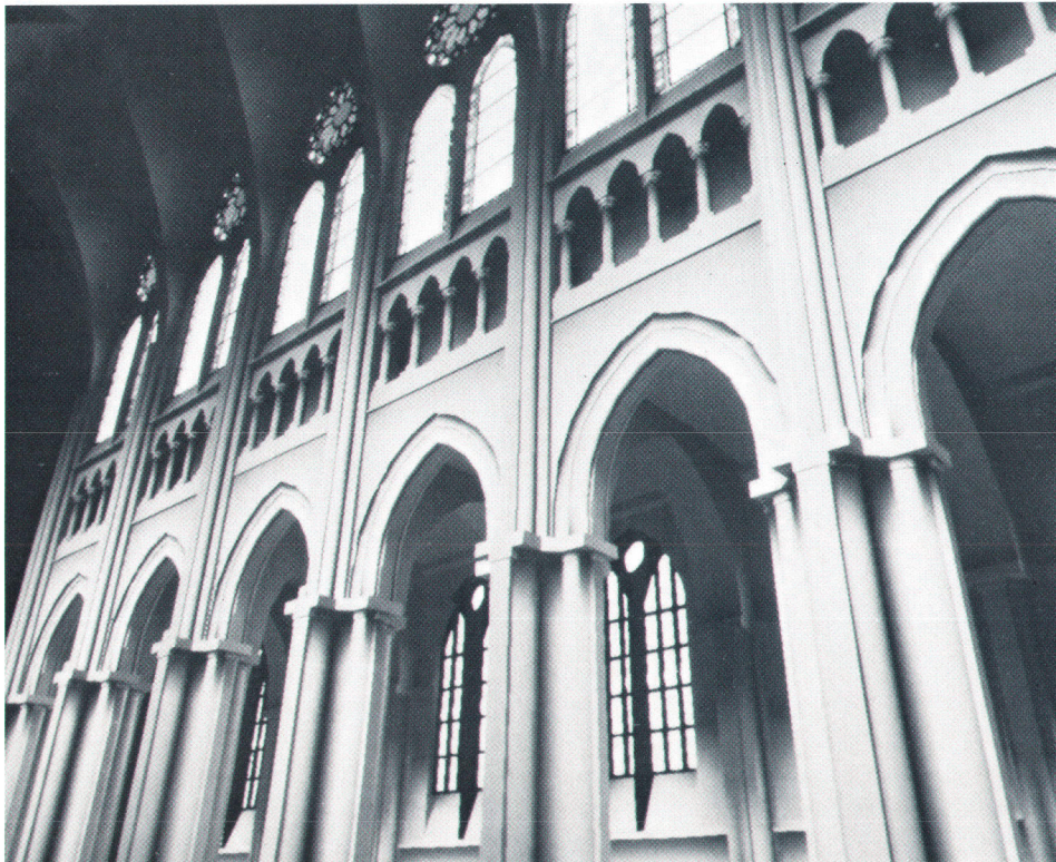
Fig. 2. This radiosity image of a cathedral with eight bays of windows and columns was done for two bays, and the remaining bays were generated by a step-and-repeat process. It took 7 minutes of preprocessing on an HP 9000 Model 350 to build the data base and subdivide the polygons (meshing), and 12 minutes per step for 40 steps (using progressive refinement) to generate the image (5 minutes and 8 minutes, respectively, on an HP 9000 Model 370). There are 9916 polygons (14,316 after meshing), 26 area lights, and four point lights.
